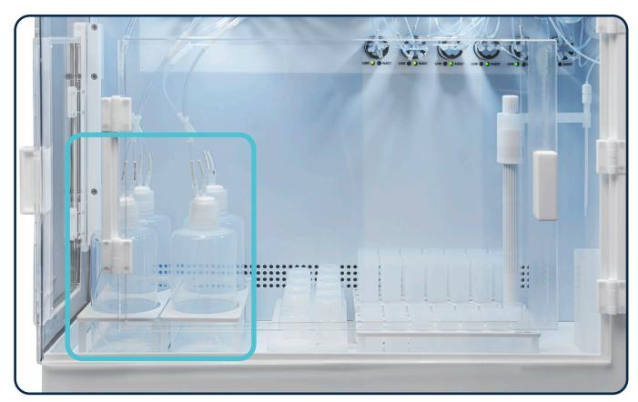
Layout of four 1L enclosed bottle samples to the left of the autosampler.
