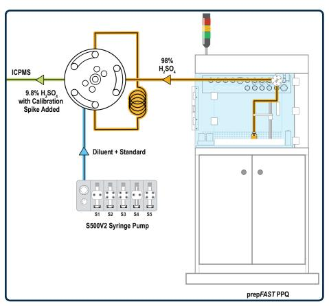
The prepFAST PPQ allows dilution by volume or weight for IPA and H<sub>2</sub>O<sub>2</sub> in concentration mode, and all semiconductorgrade chemicals in direct analysis mode. Metals are quantified using automated inline MSA or external calibration. Automated direct analysis of concentrated chemicals eliminates sample contamination caused by manual dilution into a secondary container.
